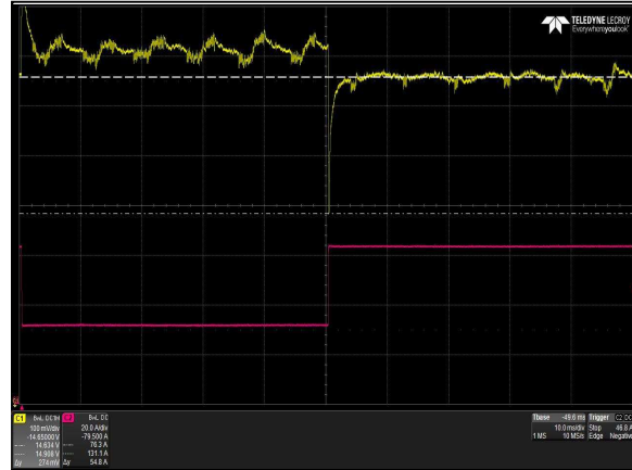
Figure 20: LCM1000N-T-4 Transient Response – V_o Deviation (high to low) 100% to 50% load change, 1A/uS slew rate, V_{IN} = 90\text{Vac} Ch 1: V_o Ch 2: I_o
