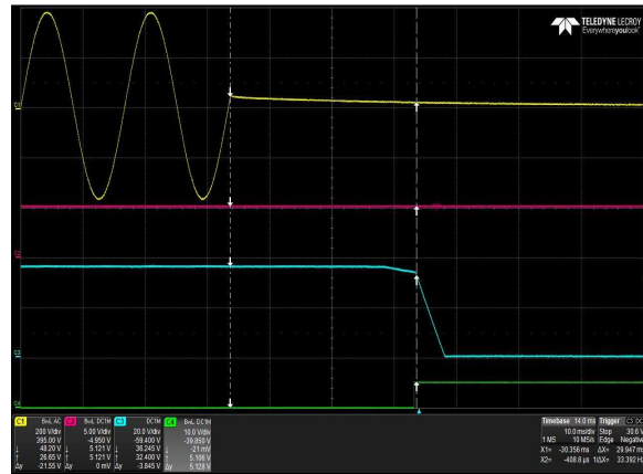
Figure 38: LCM1000U-T-4 Hold-up time – V_{IN} = 264Vac / 47Hz / 0^\circ Full Load: I_O = 27.8A (36V), I_{SB} = 1A (5V) Ch 1: V_{IN} Ch 2: V_{SB} Ch 3: V_O Ch 4: G_DCOK_C
