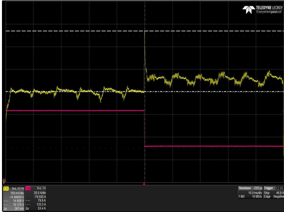
Figure 19: LCM1000N-T-4 Transient Response – V_o Deviation (low to high) 50% to 100% load change, 1A/uS slew rate, V_{IN} = 90\text{Vac} Ch 1: V_o Ch 2: I_o
