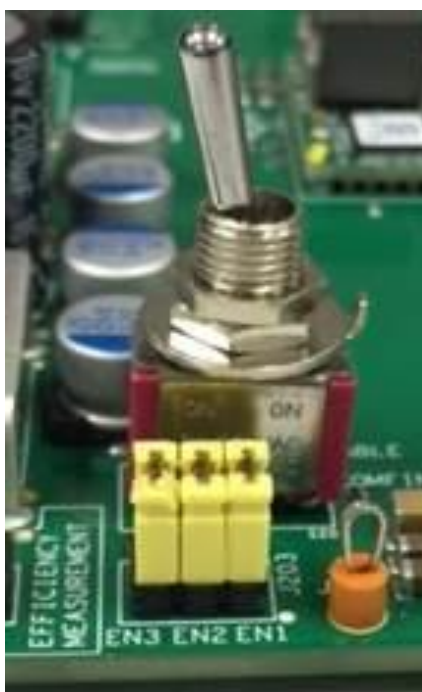
Fig. 4 – Enable jumper location and population
