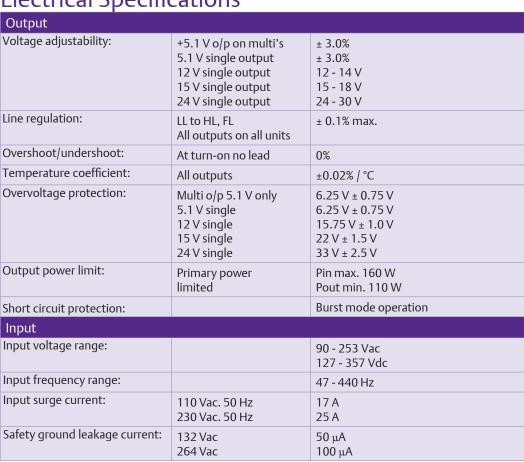
All specifications are typical at nominal input, full load at  $25\,^{\circ}\mathrm{C}$  unless otherwise stated
