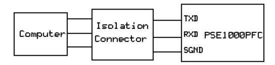
Note: Don't connect PSE1000PFC to computer directly. Please isolate the PSE1000PFC and computer with communication ports with optocouplers.
