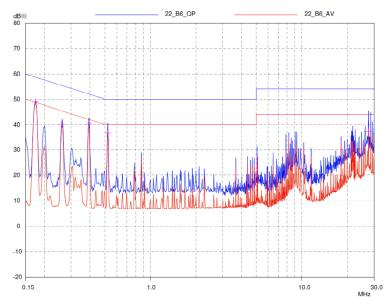
The PSE1000PFC and PSE1000DCDC-12V power supplies with external EMI filters before PSE1000PFC to ensure the convertors' conducted EMI levels comply with EN55022 (FCC Part 15) Class B and EN55022 (CISPR 22) Class B limits. The EMI measurements are performed with resistive loads at maximum rated loading.
