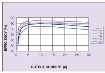
Figure 2 - Efficiency vs Load Current Vin = 3.3 V (See Note B)
