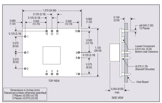
Figure 4 - Plated Through-Hole Mechanical Drawing
