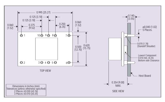
Figure 1 - Plated Through-Hole Mechanical Drawing
