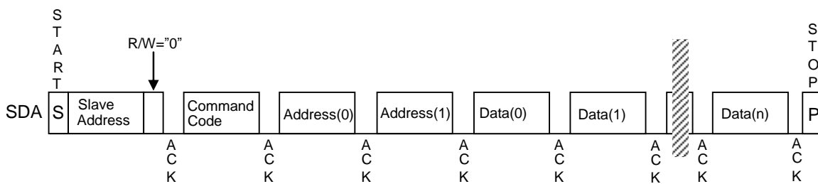
Figure 36. Data Transfer Sequence in I 2 C-bus Mode
