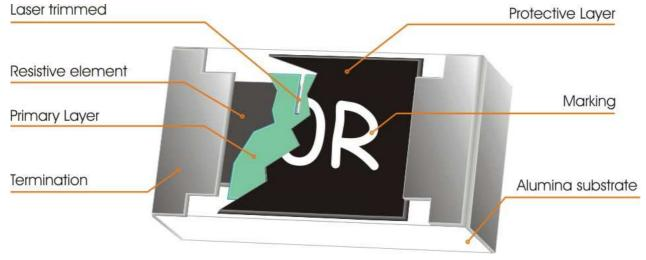
Fig 1. Construction of Chip-R
