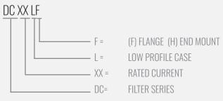
NOTE: USE ANY COMBINATION OF -X (AMPS) WITH ANY -Y RATINGS E.G. **DC100 LF**(100 AMPS, LOW PROFILE CASE, FLANGE MOUNT)
