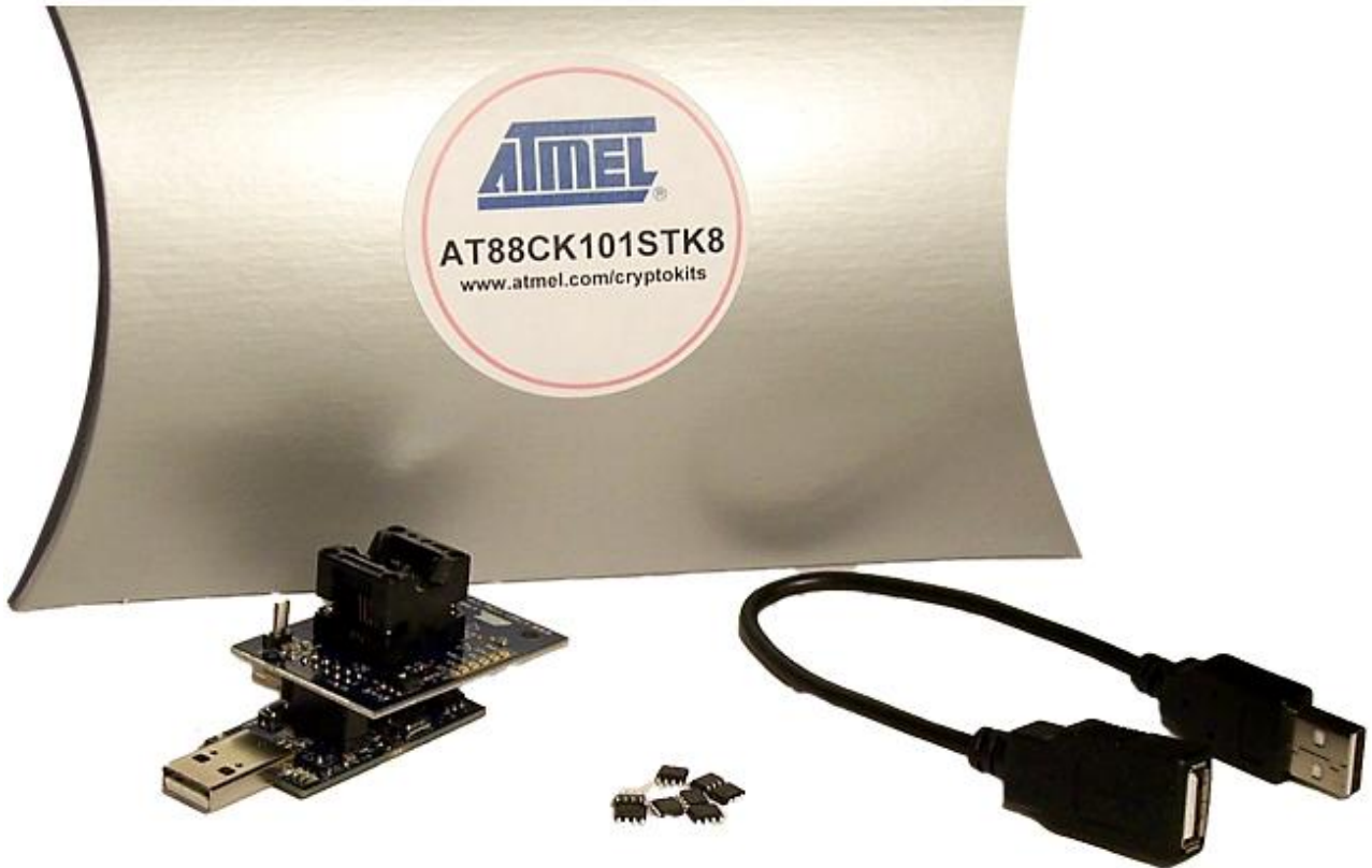
Figure 1-2. Atmel AT88CK101STK8 starter kit
