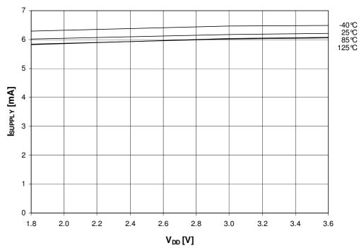
Figure 36-54. Programming Current vs. Supply Voltage V<sub>DEVDD</sub>
