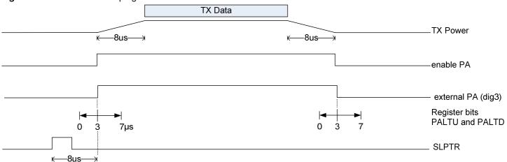
When using en external RF front-end (refer to "RX/TX Indicator" on page 97) it may be required to adjust the startup time of the external PA relative to the internal building blocks to optimize the overall PSD. This can be achieved by PARCR register in the bits PALTU/PALTD.
