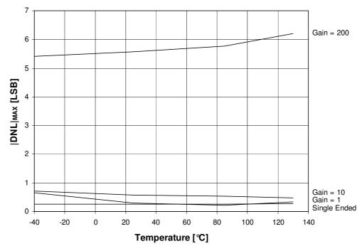
**Figure 36-40.** Differential Nonlinearity vs. Temperature at  $V_{EVDD} = 3.6V$
