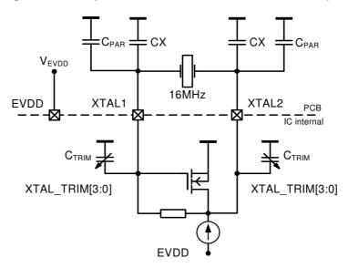
Additional internal trimming capacitors  $C_{\text{TRIM}}$  are available. Any value in the range from 0 pF to 4.5 pF with a 0.3 pF resolution is selectable using XTAL\_TRIM of register XOSC\_CTRL. To calculate the total load capacitance, the following formula can be used
