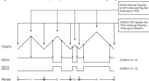
The Timer/Counter Overflow Flag (TOVn) is set at the timer clock cycle when the OCRnx Registers are updated with the double-buffered value (at BOTTOM). The OCnA or ICFn Flag is set after TCNTn has reached TOP when either OCRnA or ICRn is used for defining the TOP value. The Interrupt Flags can then be used to generate an interrupt each time the counter reaches the TOP or BOTTOM value.
