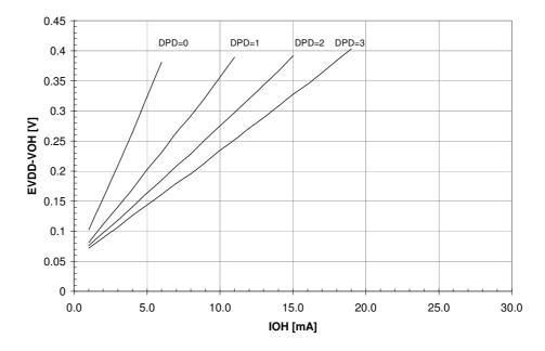
Figure 36-27. I/O Pin Output Voltage vs. Sink Current (V<sub>DD</sub>=3.0V, DPDS0 = 0)
