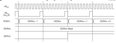
Figure 17-11 shows the setting of OCF0A and the clearing of TCNT0 in CTC mode and fast PWM mode where OCR0A is TOP.
