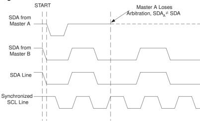
Figure 25-8. Arbitration Between Two Masters
