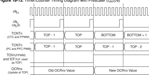
Figure 18-13. Timer/Counter Timing Diagram with Prescaler (fclkl/O/8)
