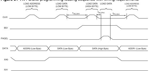
Note: 2. The timing requirements shown in Figure 31-10 above (i.e., t<sub>DVXH</sub>, t<sub>XHXL</sub>, and t<sub>XLDX</sub>) also apply to loading operation.
