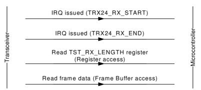
Critical protocol timing could require starting the Frame Buffer read access after the TRX24\_RX\_START interrupt. The first byte of the frame data can be read 32  $\mu s$  after the TRX24\_RX\_START interrupt. The application software must ensure to read slower than the frame is received. Otherwise a Frame Buffer under-run occurs and the frame data may be not valid.
