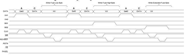
Figure 31-8. Programming the Fuses Waveforms
