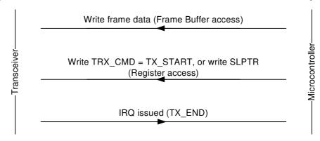
Alternatively a frame transmission can be started first, followed by the Frame Buffer write access (PSDU data) as shown in Figure 9-30 below. This is applicable for time critical applications.
