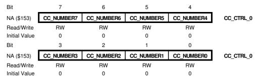
This register controls the frequency of the transceiver PLL. CC\_CTRL\_0 and CC\_CTRL\_1 form a 16 bit register. Changed CC\_CTRL\_1 bits are updated only when writing to CC\_CTRL\_0.
