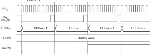
Figure 21-11 below shows the setting of OCF2A and the clearing of TCNT2 in CTC mode.
