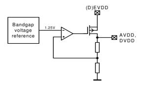
The voltage regulators require bypass capacitors for stable operation. The value of the bypass capacitors determines their settling time. The bypass capacitors shall be placed as close as possible to the pins and shall be connected to ground with the shortest possible traces.
