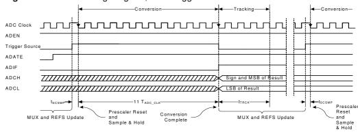
Figure 27-7. ADC Timing Diagram, Auto Triggered Conversion
