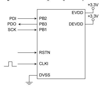
Notes: 1. If the device is clocked by the internal Oscillator, it is not required to connect a clock source to the CLKI pin.
