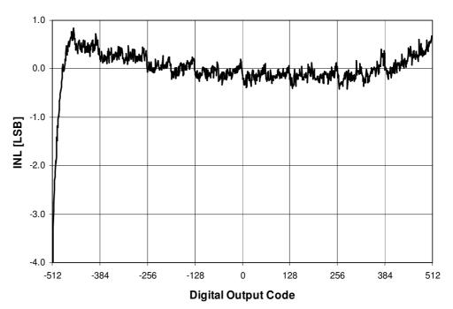
Figure 36-36. Integral Nonlinearity vs. Output Code (with PGA, Gain=10, 3.0V, 25 ℃)
