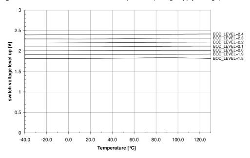
Figure 36-23. Brown-out Threshold vs. Temperature (Falling Supply Voltage)
