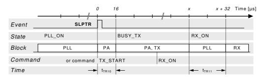
Starting from PLL\_ON state it is assumed that the PLL is already locked. A transmission is initiated either by writing "1" to bit SLPTR or by command TX\_START. The PLL settles to the transmit frequency and the PA is enabled.
