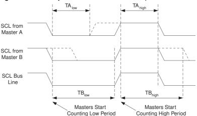
Figure 25-7. SCL Synchronization Between Multiple Masters
