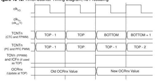
Figure 18-12. Timer/Counter Timing Diagram, no Prescaling
