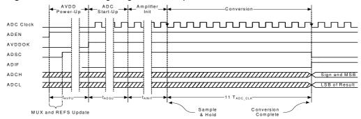
All bits of register ADCSRC are single buffered (2) through a temporary register to which the CPU has random access. This ensures that start-up time and track-and-hold time changes only take place at a safe point during the conversion. This mechanism is identical to changing an ADC channel of reference voltage, see section "Changing Channel or Reference Selection" on page 451 for details.
