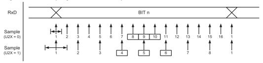
The decision of the logic level of the received bit is taken by doing a majority voting of the logic value to the three samples in the centre of the received bit. The centre samples are emphasized on the figure by having the sample number inside boxes. The majority voting process is done as follows:
