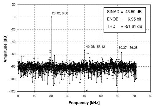
Figure 36-44. 2048 Point FFT Output for a Gain=10 ADC Channel (3.0V, 25 °C)
