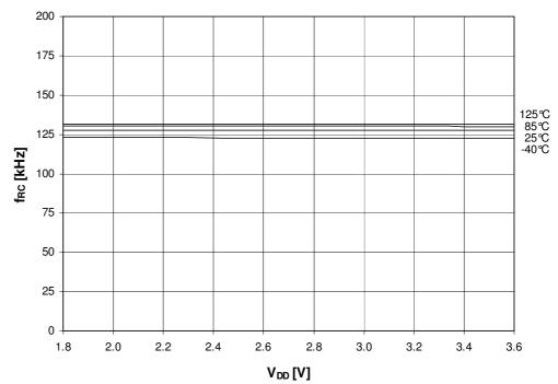
Figure 36-51. 128 kHz RC Oscillator Frequency vs. Supply Voltage
