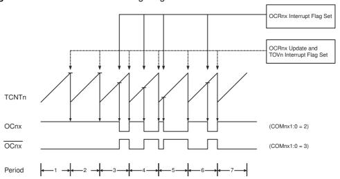
The Timer/Counter Overflow Flag (TOV0) is set each time the counter reaches TOP. The interrupt handler routine can be used for updating the compare value if the interrupt is enabled.
