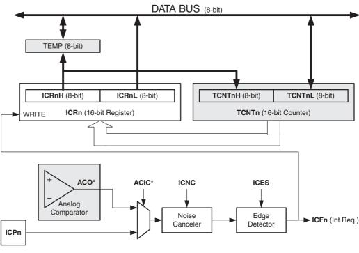
Figure 18-3. Input Capture Unit Block Diagram
