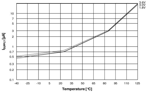
Figure 36-31. Power-Down Current vs. Supply Voltage (Watchdog Disabled)
