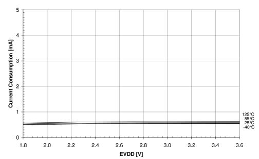
Figure 36-8. Idle Supply Current vs.  $V_{DD}$  ( $f_{CLK} = 1MHz$ ; PRR0/1 = 0xFF/0x3F)
