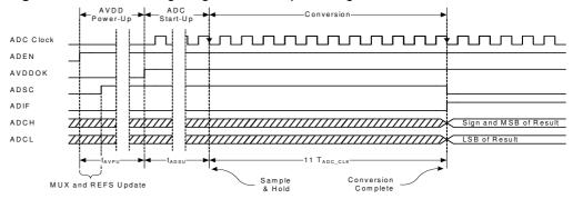
Figure 27-5. ADC Timing Diagram, Start-Up for Differential Channels
