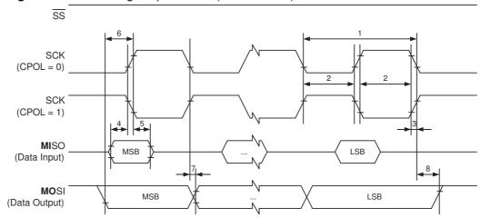
Figure 35-3. SPI timing Requirements (Master Mode)
