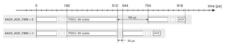
The acknowledgment time is reduced from 192  $\mu s$  to 32  $\mu s$  if bit AACK\_ACK\_TIME of register XAH\_CTRL\_1 is set.
