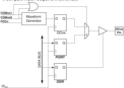
The general I/O port function is overridden by the Output Compare (OC0x) from the Waveform Generator if either of the COM0x1:0 bits are set. However the OC0x pin direction (input or output) is still controlled by the Data Direction Register (DDR) of the port pin. The Data Direction Register bit of the OC0x pin  $(DDR_OC0x)$  must be set as output before the OC0x value is visible at the pin. The port override function is independent of the Waveform Generation mode.
