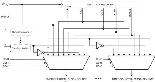
Figure 19-2. Prescaler for synchronous Timer/Counters
