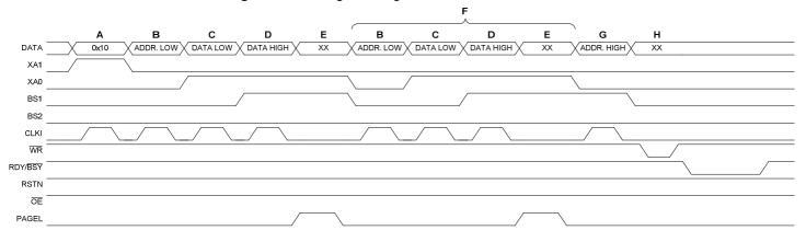
Figure 31-3. Programming the Flash Waveforms (1)
