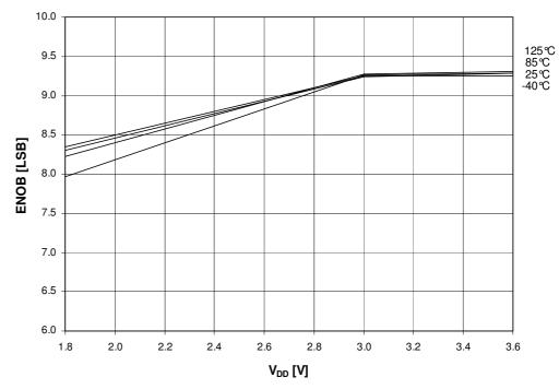
The dynamic ADC parameters for the differential channels with a gain of 10 have been measured with  $f_{ADCLK}=2$  MHz, SUT = 10, THT = 0 and an internal reference voltage of 1.6V. The input sine wave had a frequency of  $f_{IN,SIN}=20.124$  kHz and peak-to-peak amplitude of  $V_{IN,PP}=0.31V$ .
