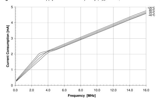
Figure 36-11. Active Supply Current vs. Frequency ( $V_{DD} = 3.0V$ , PRR0/1 = 0xFF/0x3F)
