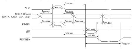
Figure 31-11. Parallel programming loading sequence with timing requirements (2)
