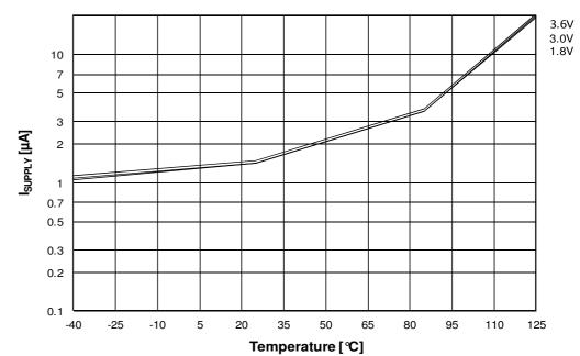
Figure 36-32. Power-Down Current vs. Temperature (Watchdog Enabled)
