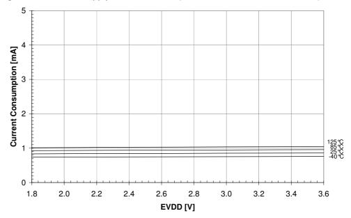
Figure 36-7. Active Supply Current vs.  $V_{DD}$  ( $f_{CLK} = 16MHz$ , PRR0/1 = 0x00/0x00)
