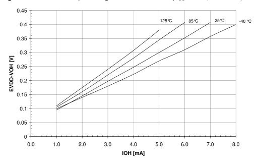
Figure 36-25. I/O Pin Output Voltage vs. Source Current (25°C, DPDS0=0)
