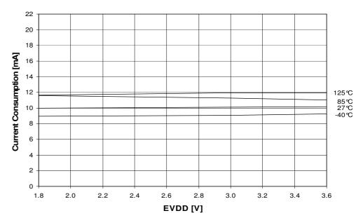
Figure 36-16. RX\_ON State Supply Current vs.  $V_{DD}$ , RPC Enabled
