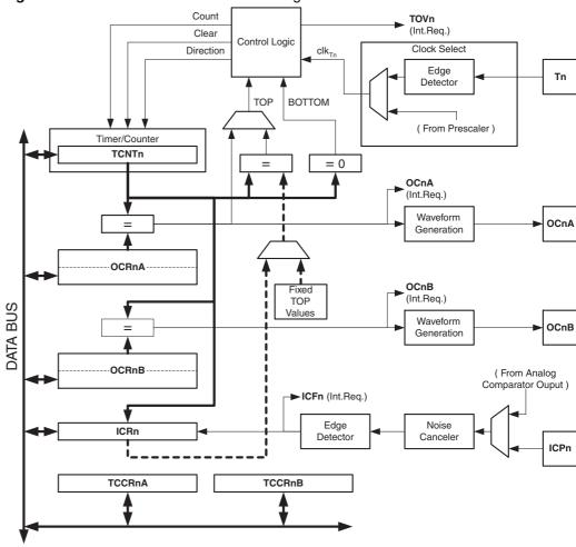
Figure 18-1. 16-bit Timer/Counter Block Diagram<sup>(1)</sup>
