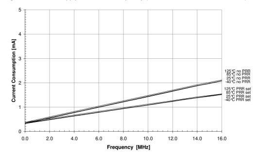
Figure 36-12. Idle Supply Current vs. Frequency (V<sub>DD</sub> = 3.0V, PRR0/1 set and reset)
