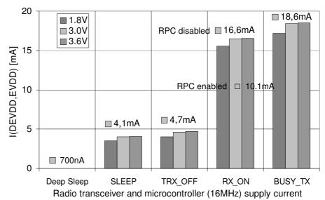
Figure 3-2 Radio transceiver and microcontroller (16MHz) supply current
