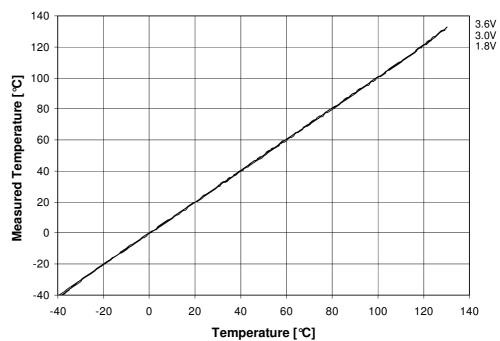
Figure 36-47. Measured Temperature Value vs. Temperature and  $V_{\text{EVDD}}$
