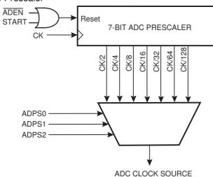
The ADC module contains a prescaler, which generates an acceptable ADC clock frequency from any CPU frequency above 100 kHz. The pre-scaling is set by the ADPS bits in ADCSRA. The prescaler starts counting from the moment when the ADC is enabled. The prescaler keeps running for as long as the ADEN bit is set, and is continuously reset when ADEN is low.
