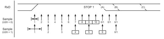
The same majority voting is done to the stop bit as done for the other bits in the frame. If the stop bit is registered to have a logic 0 value, the Frame Error Flag (FEn) will be set.
