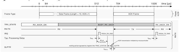
If bit AACK\_ACK\_TIME of register XAH\_CTRL\_1 is set, an acknowledgment frame can be sent already 2 symbol times after the reception of the last symbol of a data or MAC command frame.
