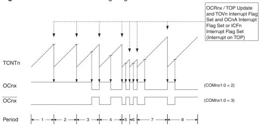
The Timer/Counter Overflow Flag (TOVn) is set each time the counter reaches TOP. In addition the OCnA or ICFn Flag is set at the same timer clock cycle as TOVn is set when either OCRnA or ICRn is used to define the TOP value. If one of the interrupts are enabled, the interrupt handler routine can be utilized for updating the TOP and compare values.
