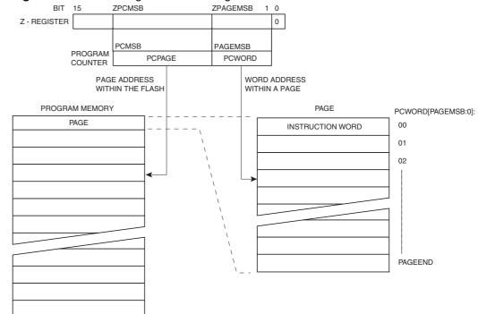
Figure 30-3. Addressing the Flash during SPM
