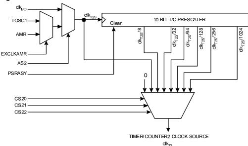
The register ASSR defines the clock source for the asynchronous Timer/Counter2. The clock source for Timer/Counter2 is named  $clk_{T2S}$ .  $clk_{T2S}$  is by default connected to the main system I/O clock  $clk_{I/O}$ . By setting the AS2 bit in ASSR, Timer/Counter2 is asynchronously clocked either from the TOSC1 or from the AMR pin. This enables the use of Timer/Counter2 as a Real Time Counter (RTC).
