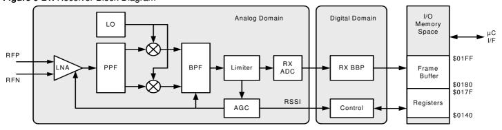
The differential RF signal is amplified by a low noise amplifier (LNA), filtered (PPF) and down converted to an intermediate frequency by a mixer. Channel selectivity is performed using an integrated band pass filter (BPF). A limiting amplifier (Limiter) provides sufficient gain to overcome the DC offset of the succeeding analog-to-digital
