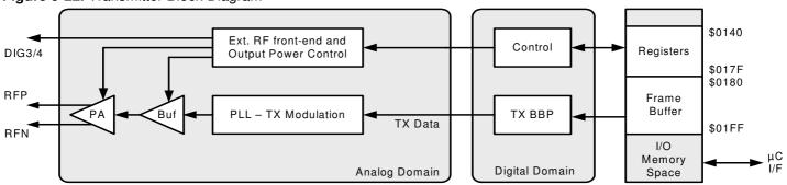
The TX BBP reads the frame data from the Frame Buffer and performs the bit-to-symbol and symbol-to-chip mapping as specified by IEEE 802.15.4 in section 6.5.2. The O-QPSK modulation signal is generated and fed into the analog radio front end.
