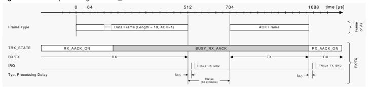
If bit AACK\_ACK\_TIME of register XAH\_CTRL\_1 is set, an acknowledgment frame is sent already 2 symbol times after the reception of the last symbol of a data or MAC command frame.
