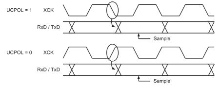
The UCPOLn bit UCRSC selects which XCKn clock edge is used for data sampling and which is used for data change. As Figure 22-3 on page 368 shows, when UCPOLn is zero the data will be changed at rising XCKn edge and sampled at falling XCKn edge. If UCPOLn is set, the data will be changed at falling XCKn edge and sampled at rising XCKn edge.
