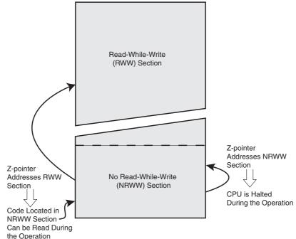
Figure 30-1. Read-While-Write vs. No Read-While-Write
