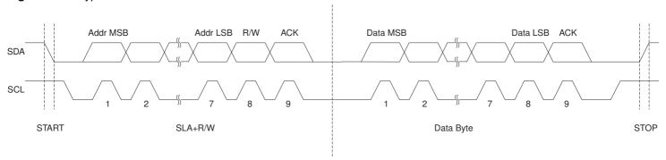
Figure 25-6. Typical Data Transmission
