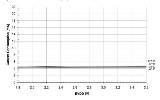
Figure 36-15. RX\_ON state supply current vs.  $V_{\text{DD}}$
