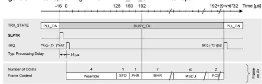
The figure above shows the timing of TRX24\_TX\_START interrupt in basic operation mode. For a description of other relevant interrupt timings see Interrupt Handling on page 42.
