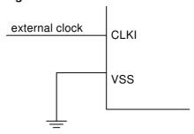
When this clock source is selected, start-up times are determined by the SUT Fuses as shown in Table 11-8 below.
