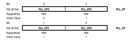
This register controls the operation of the center frequency calibration loop. Consecutive read/write commands to this register must include a wait time of at least 500ns between each access.
