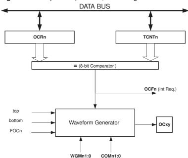
Figure 21-6. Output Compare Unit, Block Diagram
