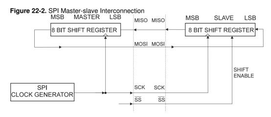
The system is single buffered in the transmit direction and double buffered in the receive direction. This means that bytes to be transmitted cannot be written to the SPI Data Register before the entire shift cycle is completed. When receiving data, however, a received character must be read from the SPI Data Register before the next character has been completely shifted in. Otherwise, the first byte is lost. In SPI Slave mode, the
