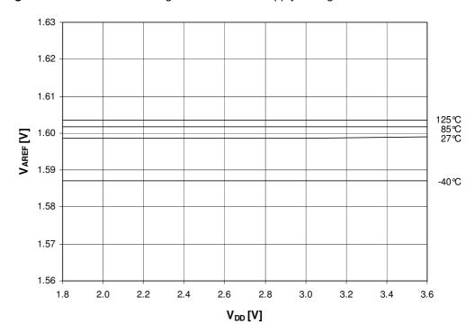
Figure 36-46. 1.6V ADC Voltage Reference vs. Supply Voltage
