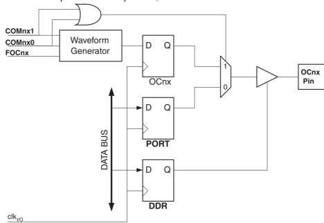
Figure 18-5. Compare Match Output Unit, Schematic
