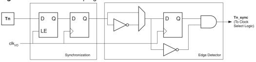
The synchronization and edge detector logic introduces a delay of 2.5 to 3.5 system clock cycles from an edge applied to the Tn pin to the counter being updated.
