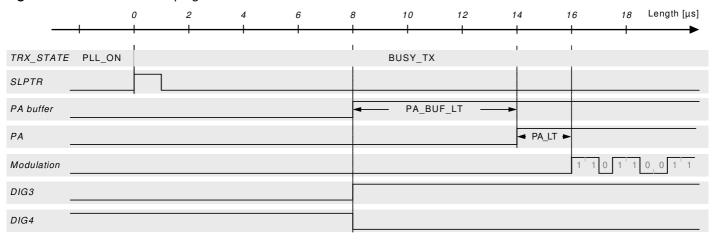
The start-up sequence of the individual building blocks of the internal transmitter is shown in the previous figure. The transmission is actually initiated by writing '1' to SLPTR. The radio transceiver state changes from PLL\_ON to BUSY\_TX and the PLL settles to the transmit frequency within 16  $\mu$ s (parameter  $t_{TR23}$  at page 46). The modulation starts 16  $\mu$ s (parameter  $t_{TR10}$  at page 46) after the SLPTR=1. The PA buffer and the internal PA are enabled during this time.
