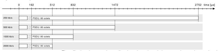
The effective data rate is smaller than the selected data rate due to the overhead caused by the SHR, the PHR and the FCS. The overhead depends further on the length of the PSDU. A graphical representation of the effective data rate is shown in the following figure:
