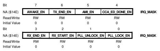
This register is used to enable or disable individual interrupts of the radio transceiver. An interrupt is enabled if the corresponding bit is set to 1. All interrupts are disabled after the power up sequence or reset. If an interrupt is enabled it is recommended to read the interrupt status register IRQ\_STATUS first to clear the history.
