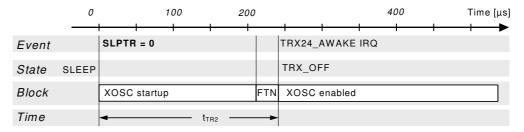
The radio transceiver SLEEP state is left by releasing bit SLPTR to "0". This restarts the XOSC if it is not already running. After  $t_{TR2}$  = 215  $\mu$ s + 25  $\mu$ s = 240  $\mu$ s (see Table 9-4 on page 46) the radio transceiver enters TRX\_OFF state. If the XOSC is already running, the radio transceiver enters TRX OFF state after 25  $\mu$ s.
