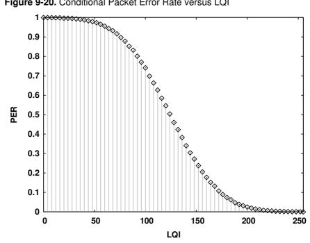
Figure 9-20. Conditional Packet Error Rate versus LQI
