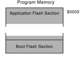
The application section of the Flash memory contains 3 user signature pages. These pages can be used to store data that should never be modified by an application program e.g. ID numbers, calibration data etc. For details see section "User Signature Data" on page 507.
