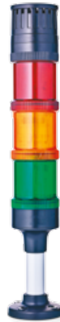
Order number: ECO60-Q81 Colours: red/orange/green Function: LED steady beacon, buzzer steady or pulsing tone Nominal voltage: 230 V AC Type of mounting: Tube mounting (100 mm tube length)
