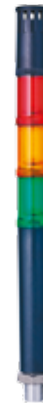
Order number: C30-Q641 Colours: red/orange/green Function: LED steady beacon, buzzer steady or pulsing tone Nominal voltage: 24 V AC/DC Type of mounting: horizontal
