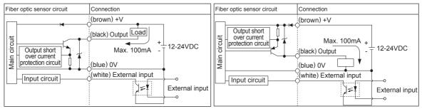
When using external input function, use photocoupler, external controller, etc. Otherwise, it may result in product damage.
