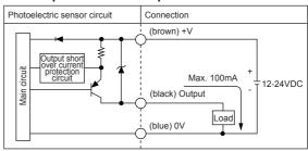
If short-circuit the control output terminal or supply current over the rated specification, normal control signal is not output due to the output short over current protection circuit.
