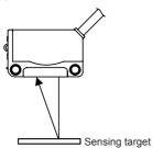
• If the sensing target has a glossy surface, mount the sensor at a 5 to 10° angle as shown in the figure. Check to see that there is no influence from background objects.
