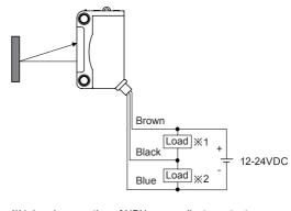
X1: Load connection of NPN open collector output
