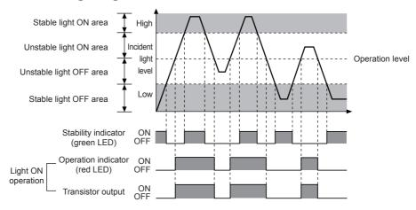
\*\*The waveforms of 'Operation indicator' and 'Transistor output' are for Light ON operation.
