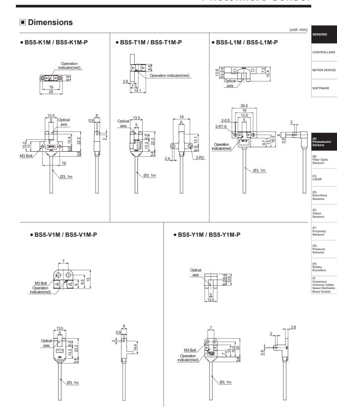
$\times$ When using photoelectric sensors closely over two units, it may result in malfunction due to mutual interference.  $\times$ When installing the product, tighten the screw with a tightening torque of 0.49N·m.
