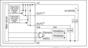
X1: PSM4: 4 of each OUT1/OUT2. PSM8: 8 of each OUT1/OUT2.
