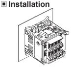
XInsert this unit into a panel, fasten bracket by pushing with tools as shown.
