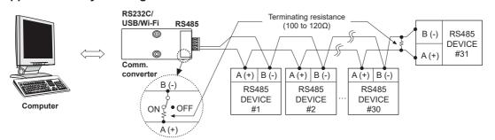
XIt is recommended to use Autonics communication converter; SCM-WF48 (Wi-Fi to RS485·USB wireless communication converter, sold separately), SCM-US48I (USB to RS485 converter, sold separately), SCM-38I (RS232C to RS485 converter, sold separately). Please use twisted pair wire, which is suitable for RS485 communication, for SCM-WF48, SCM-US48I and SCM-38I.
