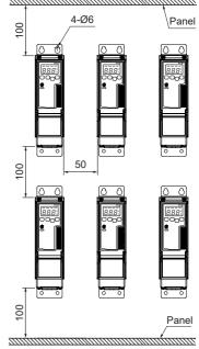
When installing multiple power controllers, please keep space at least 50mm in horizontal and 100mm in vertical between power controllers for heat radiation.
