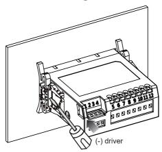
Insert the unit into a panel, fasten the bracket by pushing with tools with a (-) driver.
