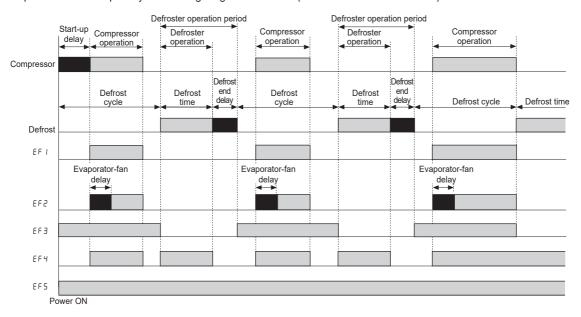
※■: Output does not turn ON but the dedicated indicator flashes at the delay period (compressor, defrost, evaporator-fan).
