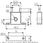
Max. load current: 80A (50/60Hz) Current ratio: 1/1000
