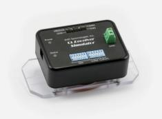
The Qi FOD Receiver is a low power receiver that can be used to test the operation and FOD performance of Qi wireless transmitters. DIP switches on top of the FOD Receiver are used to program received power offsets and to change internal loads.
