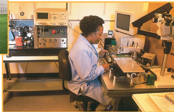
Autopacking center packages chips into waffle packs ▶
