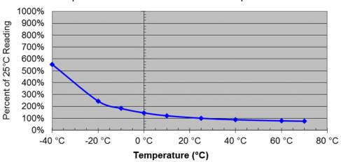
Equivalent Series Resistance vs. Temperature
