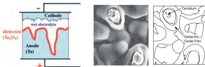
Figure 1 a. Basic Tantalum Wet Electrolytic Capacitor System
