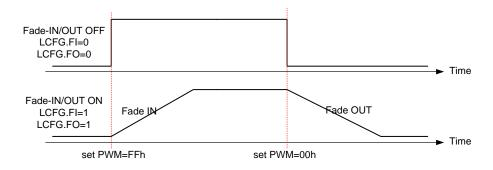
Figure 7 Fade-in/Fade-out in PWM Control Mode
