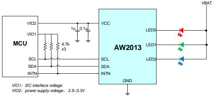
Figure 1 AW2013 Typical Application Circuit
