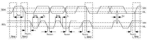
Figure 4 I2C interface timing diagram
