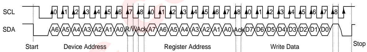
Figure 6 I 2 C Write Byte Cycle
