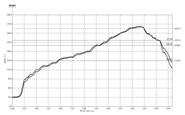
Figure 17 Package Reflow Oven Thermal Profile
