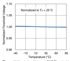
Figure 11 Normalized Internal OVP Threshold
