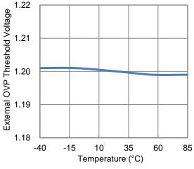
Figure 12 External OVP Threshold
