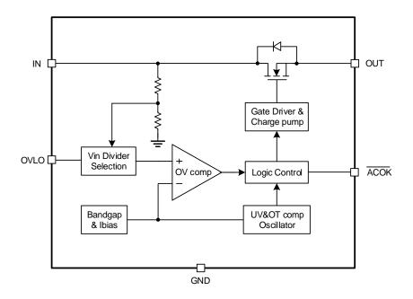
Figure 3 Functional Block Diagram
