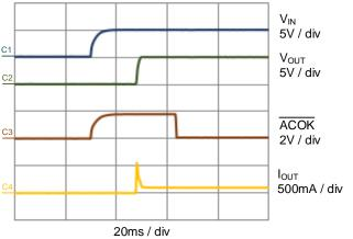
Figure 14 Power-up ( $C_{OUT} = 100 \mu F$ , 100mA load)
