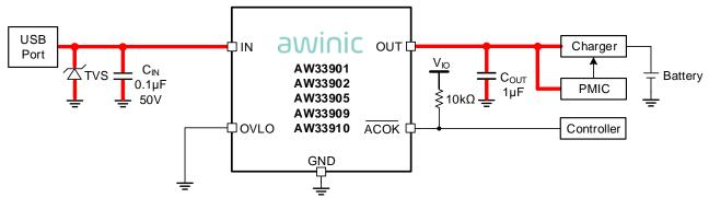
Figure 4 AW339XX typical application circuit(using default OVP threshold)
