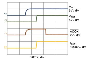
Figure 13 Power-up ( $C_{OUT} = 1\mu F$ , 100mA load).
