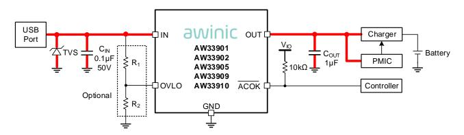
Figure 1 AW339XX typical application circuit
