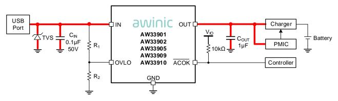
Figure 5 AW339XX typical application circuit(using external OVP threshold)
