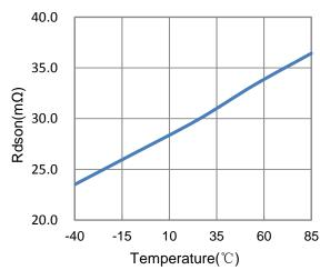
Figure 8  $R_{dson}$  vs. Temp. ( $I_{OUT} = 1A$ )
