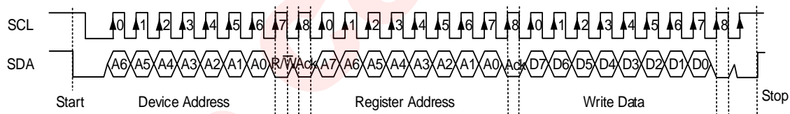
Fig 24 I 2 C Write Timing
