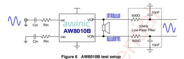
Low pass filter uses resistance and capacitor values listed in Table 1.
