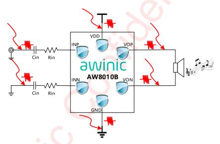
Figure 9 RF Energy Coupling Diagram
