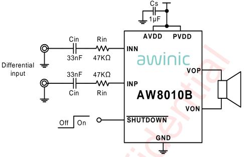
Figure 4 AW8010B Application Schematic With Differential Input
