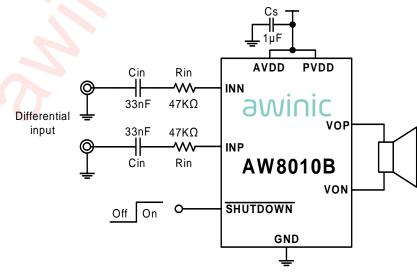
Figure 1 AW8010B Application Schematic With Differential Input
