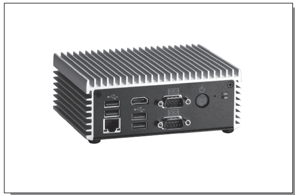
Figure 2: Axiomtek Ultra Compact Embedded System with Pico-ITX SBC - eBOX560-880-FL
