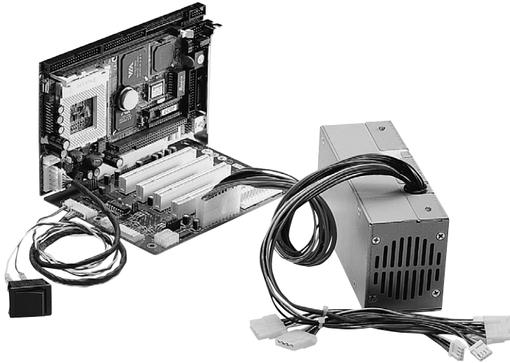
Photo 1 - Plug the ATX 20-pin male connector into the female connector of the Axiomtek backplane.
