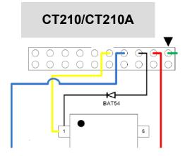
Table 4 Azoteq USB-dongle Pin Assignment for Programming IQS333 OTP Using Azoteq USBProg
