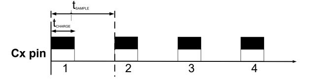
Figure 5.1 Charge cycles as can be seen on Cx.
