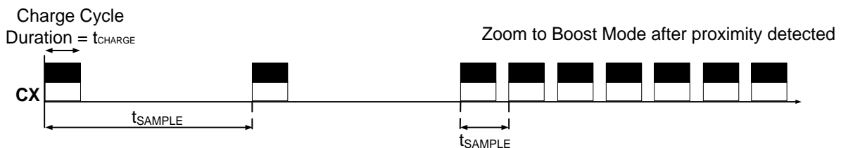
Figure 5.4: LP Modes: Charge cycles
