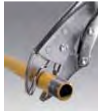
Gripping and welding pliers are used for clamping work pieces during welding and assembly work.
