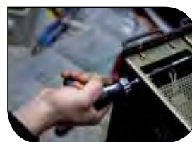
T-handle and pistol-grip for application when accessibility is a challenge.
