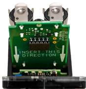
Q45 battery board
