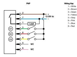
Note: Cabled wiring diagrams are shown. Quick disconnect wiring diagrams are functionally identical.
