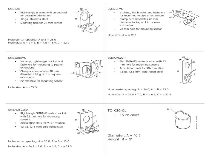
All measurements are listed in millimeters, unless noted otherwise.
