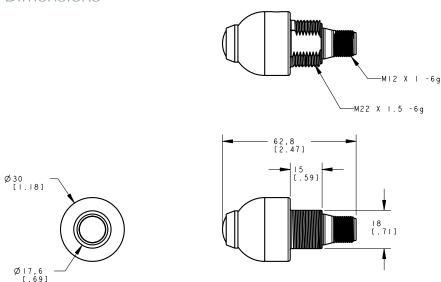
All measurements are listed in millimeters [inches], unless noted otherwise.
