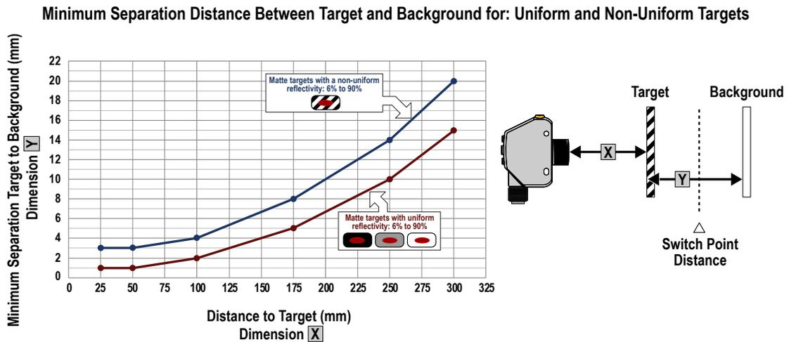
Figure 16. Minimum Object Separation Distance (90% to 6% reflectance)
