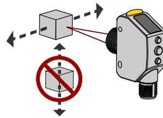
Figure 4. Optimal Orientation of Target to Sensor
