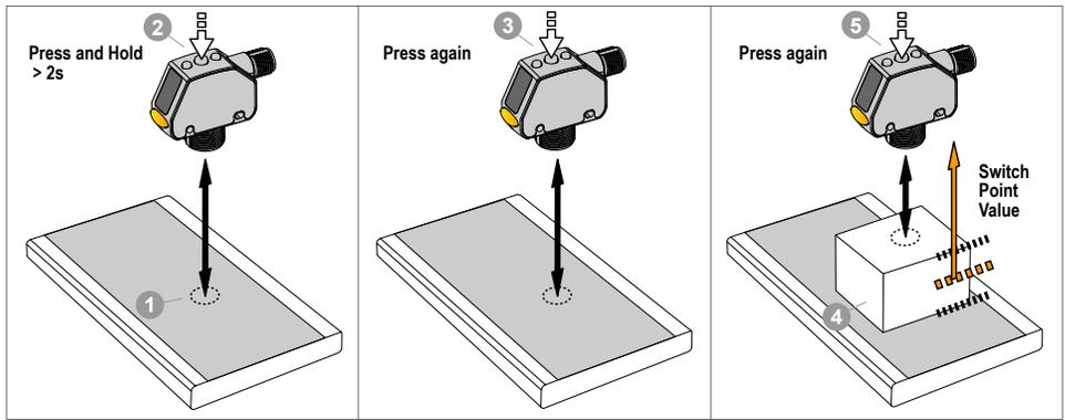
Figure 12. Two-Point Static Background Suppression (Light Operate shown)
