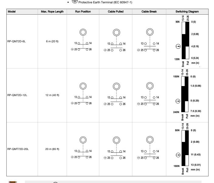
Note: This symbol of for a positive-opening safety contact (IEC 60947-5-1) is used in the switching diagram to identify the point in actuator travel where the normally-closed safety contact is fully open.
