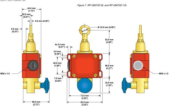
45.5 mm 20.5 mm - 5.0 mm (0.20") Ø 25.0 mm (0.98") Ø 15.0 mm (0.59") 8.5 mm (0.33") 53.0 mm (2.09") 4x 5.4 mm (0.21") — 7.5 mm (0.30") 95.5 mm (3.76") 76 mm (2.99") M20 x 1.5 -M20 x 1.5 **®** [i] **(%)** 12 mm (0.47") 33.0 mm (1.30") 72.0 mm (2.83") 69.0 mm (2.71") 82.0 mm (3.23")
