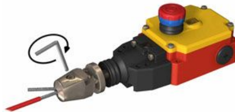
Tightening the rope into the internal turnbuckle (models RP-RM83F-..LT and -..LTE)
