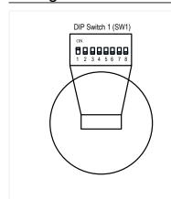
Input channel select-Use switch positions 1 through 6 on SW1, to select the channel that would be used to operate the audible module. Switch positions 7 and 8 are not used.
