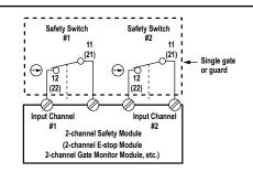
The non-safety contact (33/34) will switch at a greater degree (rotation) than the safety contacts and may not indicate if the guard is slightly open (see Figure 3 on page 2). In such situations, an unused safety contact can more accurately indicate the status of the guard.
