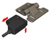
4. Lift the red plastic washer from the switch. Discard the plastic washer; it cannot be reused.
