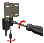
2. If you are changing the switch to the opposite side, insert a flat-blade screwdriver between the hinge housing and the plastic plug to gently pry the plastic plugs out. Retain the plastic plugs for later reuse.
