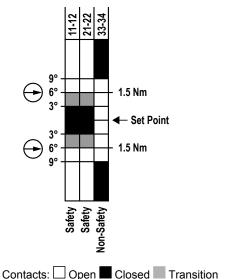
Figure 4. Contact Configuration (Gate Closed State) for Cabled Models
