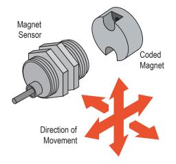
Normal Direction of Approach: movement is perpendicular to the plane of the sensing face.
