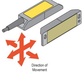
Alternate Direction of Approach: movement is parallel to the plane of the sensing face
