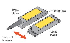
Normal Direction of Approach: movement is perpendicular to Incorrect Direction of Approach: Label to label approach of sensor and magnet is not possible
