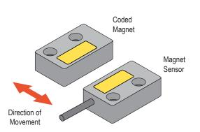
Normal Direction of Approach: movement is perpendicular to Incorrect Direction of Approach: Label to label approach of the plane of the sensing face
