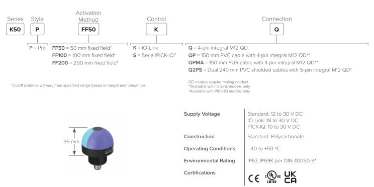
\*Cabled models also meet DIN IP69K if the cable and cable entrance are protected from high-pressure spray
