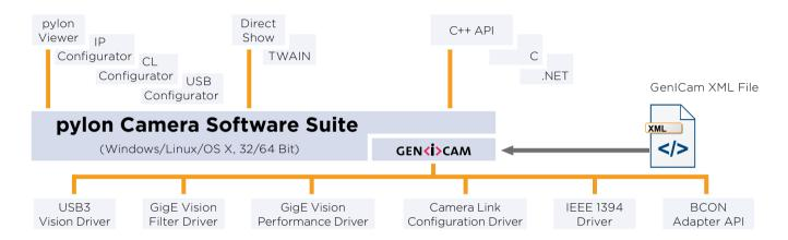
The architecture of the pylon Camera Software Suite is based on GenlCam Technology, which offers easy access to the newest camera models and the latest features. Changing an existing camera device in any application essentially becomes a plug and play process.
