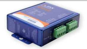
Model BB-485OPDRI-PH is a premium, heavy industrial RS-422/485 isolated repeater. Designed for rugged industrial environments, it meets some of the most exacting compliance tests in the industry. IEC 61850-3 and IEEE 1613 rated, it is suitable for installation in electrical substations. (These specifications are more stringent than NEMA TS1/TS2 requirements for transportation applications).
