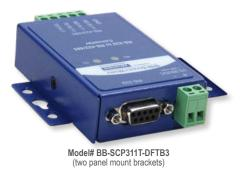
The BB-SCPx series of RS-232 to RS-422/485 converters are compact and tough, designed and tested to meet heavy industrial EMC standards. The RS-232 signal is connected via a female DB9 connector. The RS-422/485 (2-wire and 4-wire) signal is connected via a removable terminal block, making wiring easy. Bit-wise enabled circuitry automatically detects the character time-out eliminating the need to set DIP switches for the baud rate.
