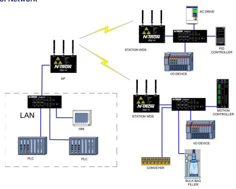
In station WDS mode, the 702-W can be connected to a remote wired Ethernet switch with multiple devices connected to the switch.
